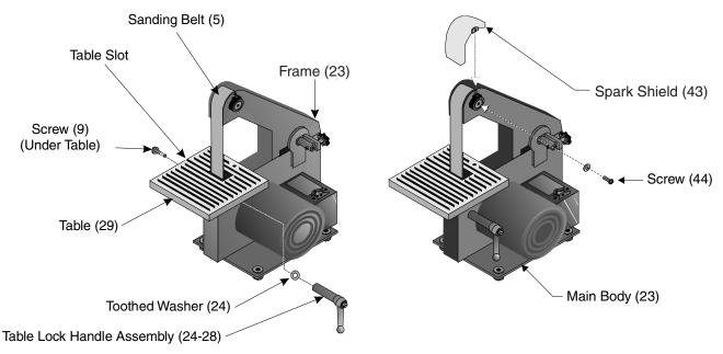
6. Loosen the Screw (44) most of the way as shown above.
